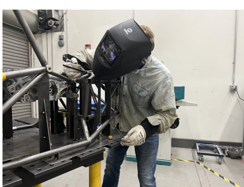
Liam preparing to run a tig seam weld on the upper shock mounting structure
